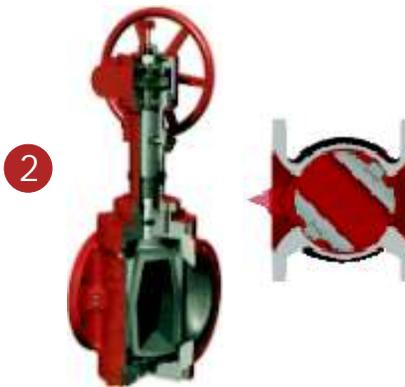
Turning the operator handwheel clockwise rotates the plug assembly 90° to block flow. During rotation, clearance is maintained between the seal and the valve body, allowing free movement and avoiding abrasion.
