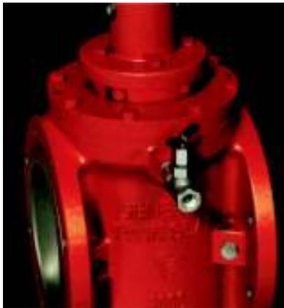
A Manual Body Bleed Valve is included on this General Twin Seal. This bleed valve installed in the body cavity is only opened after the General Twin Seal is closed. Seal effectiveness can be immediately evaluated. This bleed valve must be closed before the General Twin Seal is reopened.
