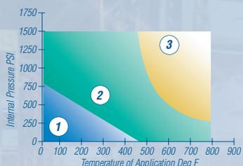
① In area one, the gasket material is suitable using common installation practices subject to chemical compatibility.
