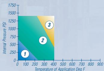
These graphs were developed from the testing of KLINGER® materials. Do not use them for competitors' materials, since non-asbestos gasketing materials do not have service equivalents.
