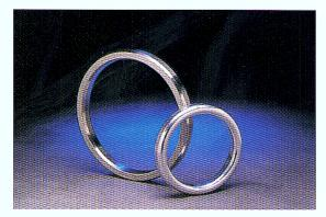
and completion equipment. However, today this product range can also be found on valves and pipework assemblies, along with some high integrity pressure vessel joints. Standard Style R Ring Joint gaskets are manufactured in accordance with both API 6A and ASME B16.20 size/ratings. Available in both oval and octagonal configurations, both types are interchangeable on the modern octagonal type grooved flanges.
