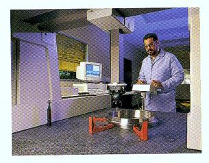
Flexitallic utilizes a state-of-the-art coordinate measuring machine (CMM) in our quality control operations. The CMM is used to verify critical dimensions on machined parts and gives Flexitallic a competitive advantage in the marketplace.
