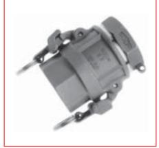
Close the coupler by rotating the cam arms towards the body of the coupler. Locking occurs when the cam arms are closed. The coupler is properly closed when the locking levers on both cam arm assemblies are flush.
