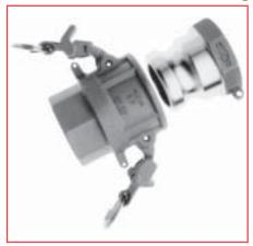
Open the coupler by pulling back on the locking lever above the cam arms while rotating the arms away from the body of the coupler.
