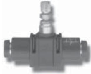
Allows air to pass in one direction while blocking flow in the other direction. A pressure of more than 7.3 PSI will overcome the spring pressure and allow flow. An arrow indicates free flow direction. Maximum Working Pressure: 145 PSI.
