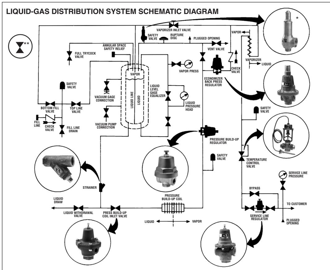
\* C-776 Cryogenic safety relief valve - For additional information, write or call for data sheet CRY-C776.
