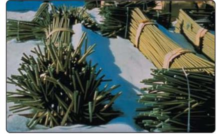
3M™ Scotchkote™ coated rebar ready for installation. 16
