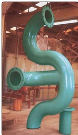
Header piping for a water purification plant illustrates the types of complex shapes that can be coated with 3M™ Scotchkote™ coating. 1
