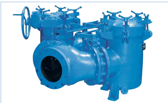
For higher flow rates that require a duplex strainer, the large-size Model 50 switches flow between baskets with a built-in butterfly valve. This design is also compact and can be important when space is at a premium. Available in 10" to 18" sizes.
