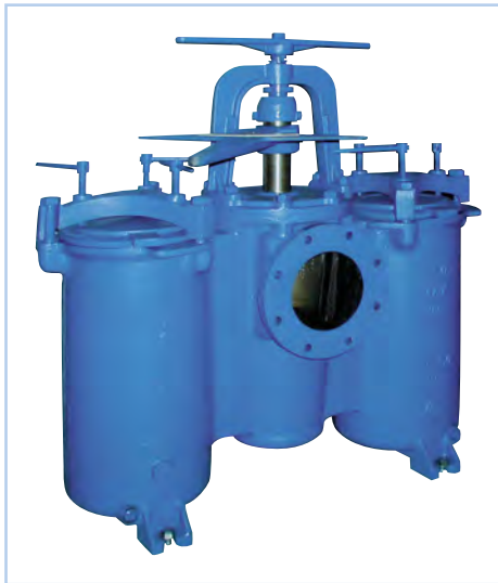
The Model 50 duplex strainer is for 5", 6" and 8" pipelines where the process cannot be shut down for basket changeout. A tapered plug is used to divert flow from one basket to the other.
