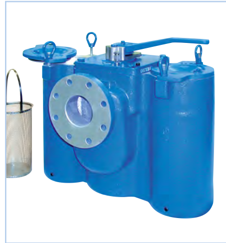
Model 53BTX ball-type strainer, in sizes from 3/4" to 4", uses a dynamic ball sealing system which keeps the out-of-service strainer basket chamber from filling with fluid while the basket is being changed. A unique diverter cartridge is easy to remove for service.
