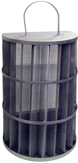
By convoluting (pleating) the strainer element, the screening area is increased while reducing the total basket size
