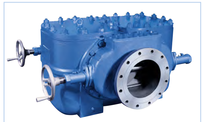
For handling very large volumes of water, and for quick and easy basket changeout, the Model 570 includes 4 baskets per chamber. Flow is switched by a sliding gate mechanism operated by a hand wheel. Available in sizes from 8" to 36".
