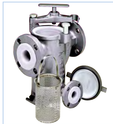
Model 72L Tefzel®-Lined Simplex Strainer for Pipelines from 1" to 6". This is a low-cost alternative to exotic alloy strainers for a wide variety of corrosive or abrasive lined piping applications.
