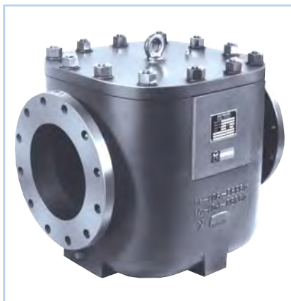
Model 510 Multibasket Simplex Strainer for Pipelines from 8" to 36". Extremely rugged with a low profile for tight installations. Angled baskets permit a high flow rate and a low pressure drop.
