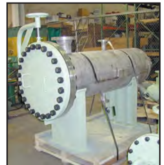
Custom-fabricated Model 90 stainless steel simplex strainer with davit to aid in cover removal and basket changing.
