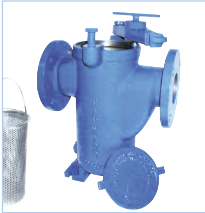
Model 72 Simplex Strainer for Pipelines to 8". Unusually large basket capacity...a free-straining area of at least 6 times the pipe cross-sectional area.
