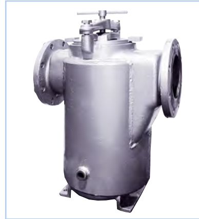
Model 72SJ Steam-Jacketed Simplex Strainer for Pipelines to 8". Use for materials that must be kept hot in order to remain fluid. Cover seal can be Viton® or other non-asbestos material for higher temperatures.
