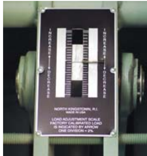
Load adjustment scale shown applies to size 1 through 83 only. The load adjustment scale for sizes 84 through 110 1 division equals 1%
